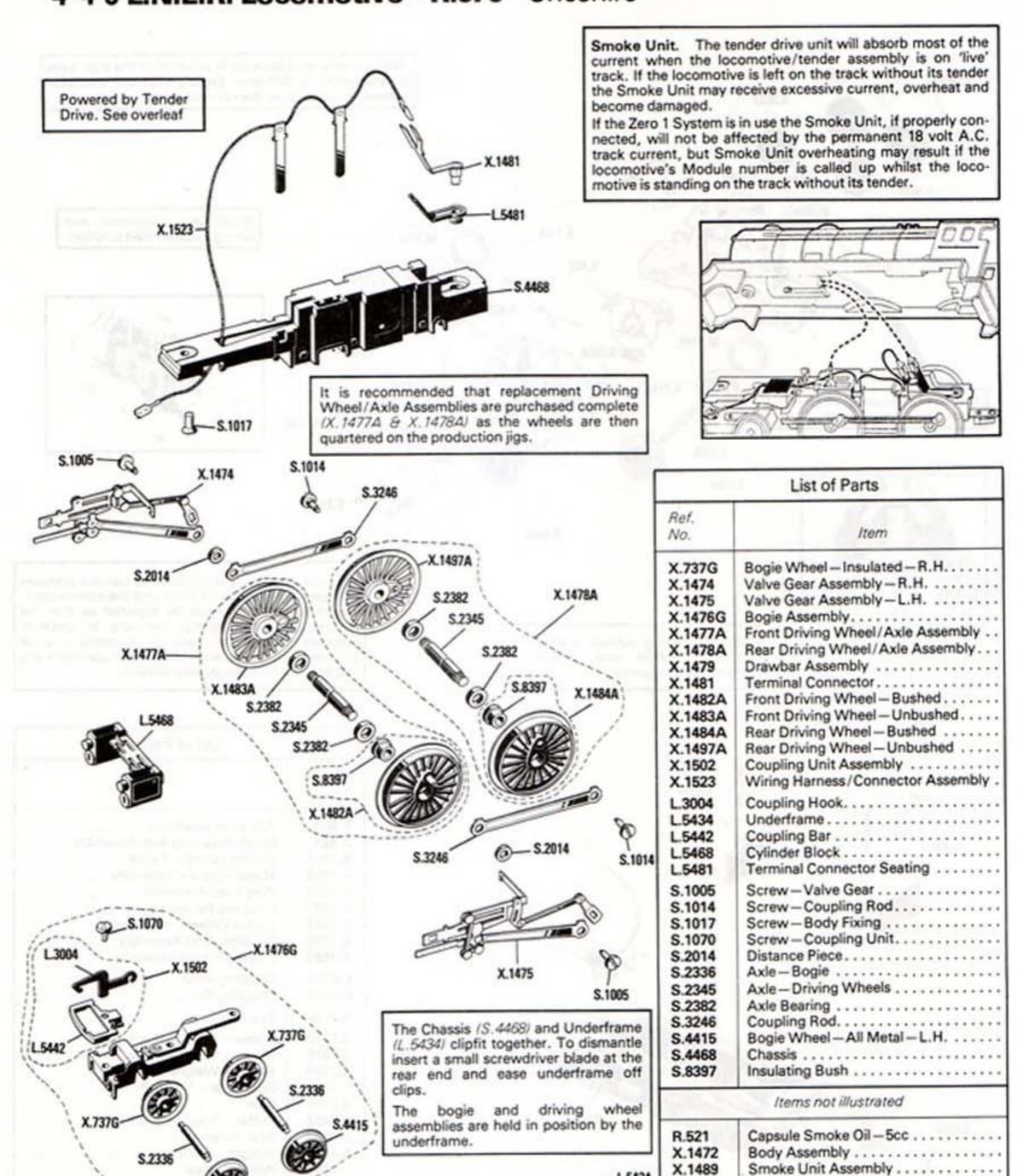
When Locomotive and Tender are coupled the contact pin on the Tender must be firmly pressed down so that it passes through the spring contact underneath the Locomotive Drawbar.
